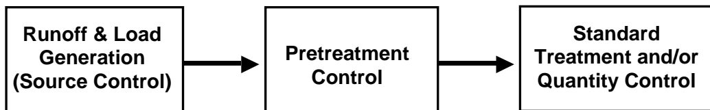
Figure 3-6 Generalized Stormwater Treatment Train
